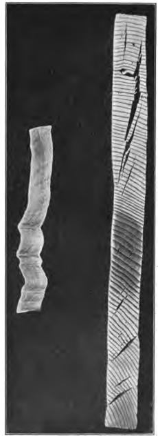
Fig. 68.—Cross section of cedar (on left) and redwood boards (on right) showing collapse and bulge respectively, in very wet lumber dried at a high temperature.
